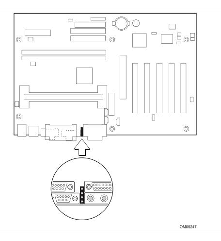
Figure 19. Enhanced Diagnostic LEDs
